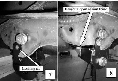
insert the bolt. Once in, rotate the spring back and insert the lower shackle bolt in the rear hanger. Torque the front spring hanger bolt to **95 ft lb**; leave the rear shackle bolt loose it will be tightened after the vehicle has been set down.
